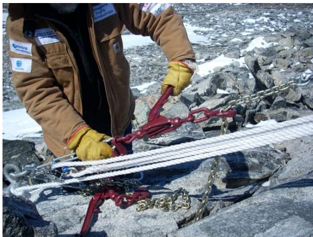
Tightening the chain tensioner
