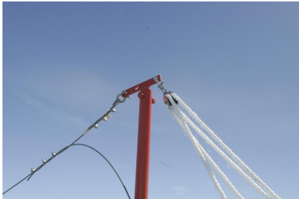
Short 'twig' of cable attached to the gin pole
