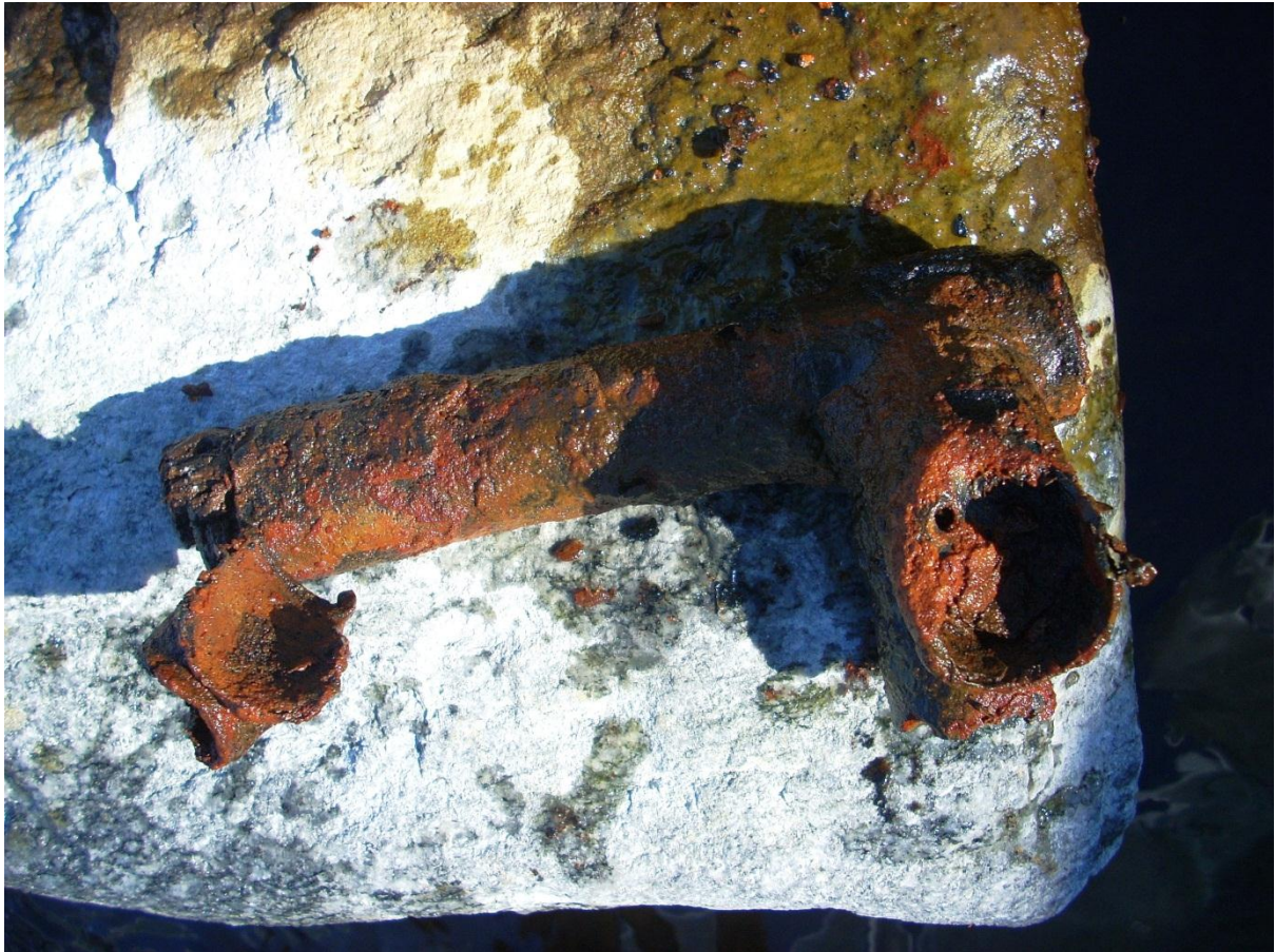
Fragment 3: Straight part from the bottom of the diamond-shaped frame section. It can be seen that a wooden dowel was inserted in the Left hand end, and subsequently cut off , and that there is a round section on top of that end, probably the remnants of a socket for the tail assembly.
