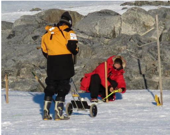
Tony Stewart performs a magnetometer survey. The recording head is in the non-ferrous cart, and Jody Steele holds the tape to provide accurate sampling distances.
