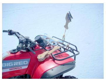
The kite string is anchored to the front rack of the quad bike via a double cleat on a board. The winder is the blue device seen on the left hand side of the rack, and the pulley to bring the kite down on the right.
