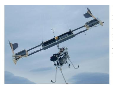
The camera rig consists of a C channel of carbon fibre containing triggering electronics, and two camera housings at the end of 1m carbon fibre rods. Tail fins stabilise the rig in yaw and pitch. The rig is suspended on a Picavet suspension which helps keep it vertical.
