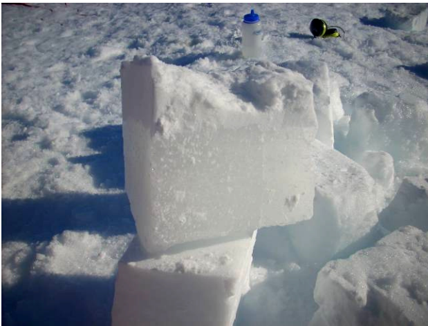
Figure 25 Layer of clear hard ice encountered at about 1.25m which is shown on the radar scan (Figure 22:) and at a depth consistent with the ice level estimated from pictures of the 2002 melt.
